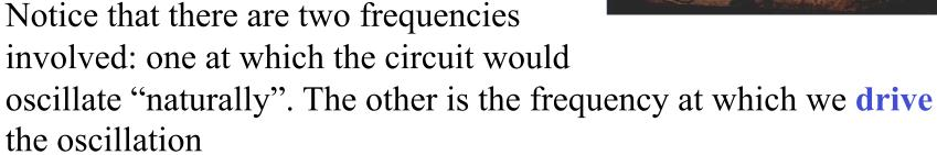
However, the "natural" oscillation usually dies off quickly (exponentially) with time. Therefore in the long run, circuits actually oscillate with the frequency at which they are driven. (All this is true for the gentleman trying to make the lady swing back and forth in the picture too).
