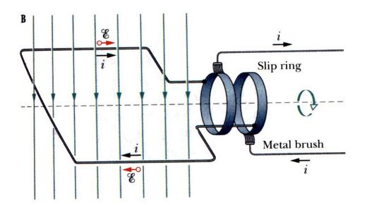
We have studied that a loop of wire, spinning in a constant magnetic field will have an induced emf that oscillates with time,
