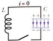
Capacitor initially charged. Initially, current is zero, energy is all stored in the capacitor.
