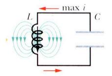
Capacitor discharges completely, yet current keeps going. Energy is all in the inductor.
