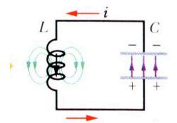
$$\frac{dE_{tot}}{dt} = 0 = \frac{1}{2}L\left(2i\frac{di}{dt}\right) + \frac{1}{2C}\left(2q\frac{dq}{dt}\right) \qquad i = \frac{dq}{dt}$$
