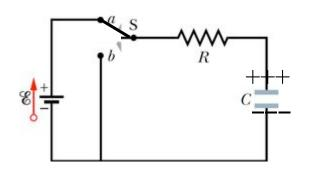
Assume the switch has been closed on a for a long time: the capacitor will be charged with Q=CE.
