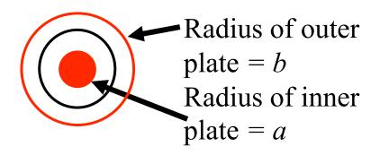
Concentric spherical shells: Charge +Q on inner shell, -Q on outer shell
